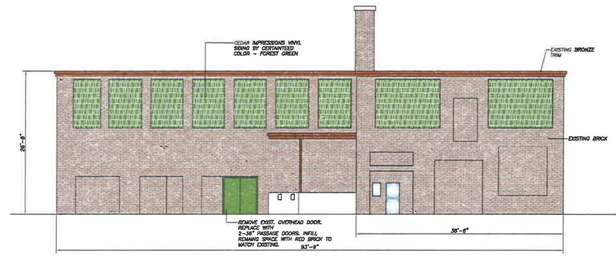
SOUTH ELEVATION SCALE: 1/8" = 1'
