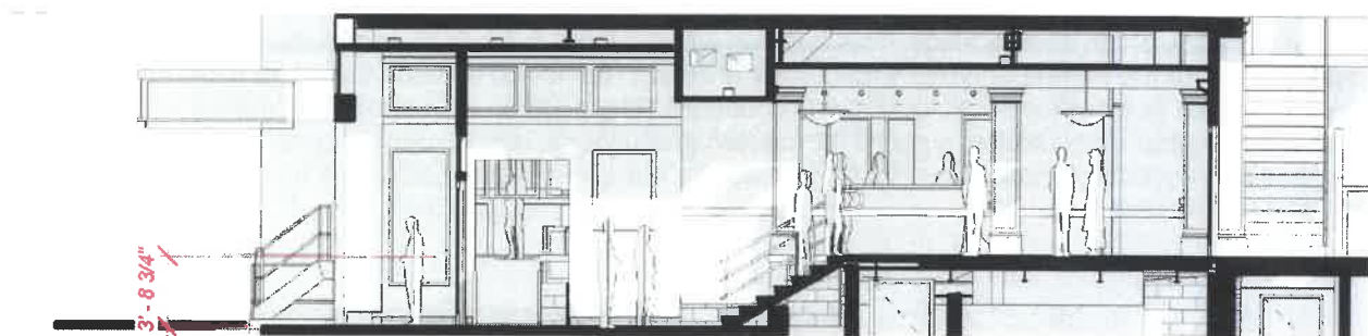
Figure 5 - Proposed Lobby provide level access to wheelchair lift and then to elevator
