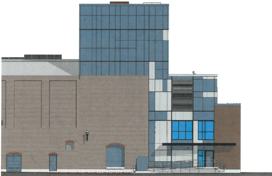
Figure 13 – North Elevation of Addition to Stagehouse
