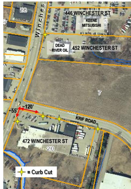
The above image displays the approximate locations of curb cuts for the property at 472 Winchester St and also for the shared curb cut at 452 Winchester St/446 Winchester St. The arrows in red indicate the approximate distances of select curb cuts from the intersection of Winchester St and Krif Rd.
