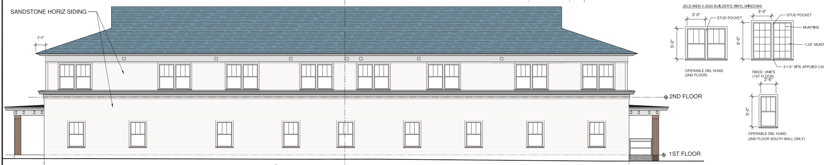
4 WEST ELEVATION scale: 3/16" = 1'-0"
