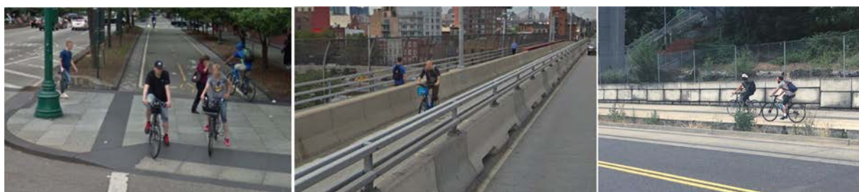
Fig. 2. Examples of protected bike lanes with heavy separation: Hudson River Greenway in Battery Park, New York (left); Pulaski Bridge, New York (center); Southwest Moody Ave, Portland (right).
