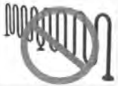
This type of rack does not support the bicycle frame in at least 2 places.
