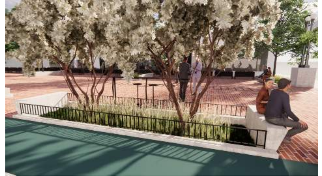
Option 2 - Vertical Granite Curb with Railing
