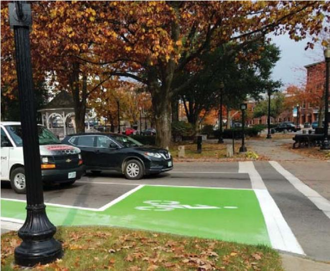
Figure 3.12. Image of a painted "bicycle box" on Central Square in Keene.
