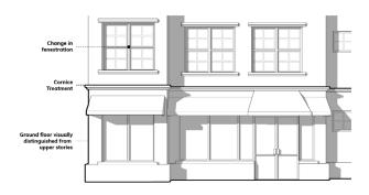
F. Buildings shall be designed with consistent building materials and treatments that wrap around all facades visible from a public right-of-way. Where material or color treatments change, there shall be a significant change in surface plane of a minimum of 6-in in difference. Differing materials are encouraged to terminate at inside corners.
