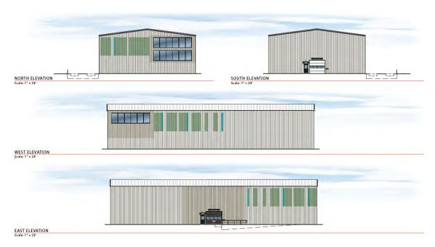
Figure 3. Image of the revised elevations for the proposed new building (not to scale).
