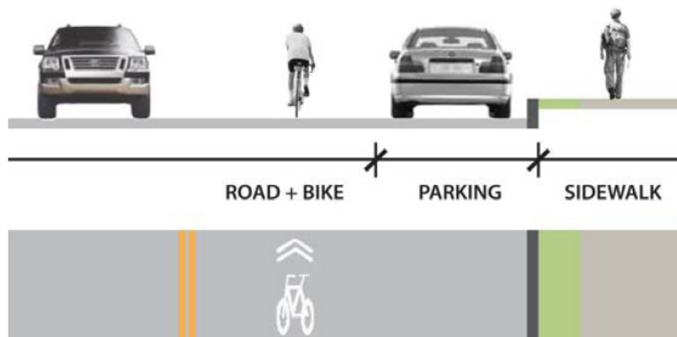
Figure 2.4 Sharrow design from FDM (Final Denver Moves, 2011)
