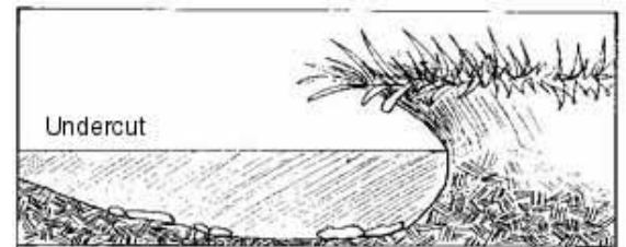
Undercut streambank, bank material has eroded below the root zone of streambank vegetation. Graphic credit: Environmental Protection Agency.
