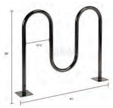
1. INSTALL 1/2" STAINLESS BOLTS INTO DROP-IN ANCHORS BY HILT. 2. SET TWO 8" SONOTUBES FILLED WITH CONCRETE TO CONNECT BASE PLATES TO. 5 - BIKE WAVE BIKE RACK
