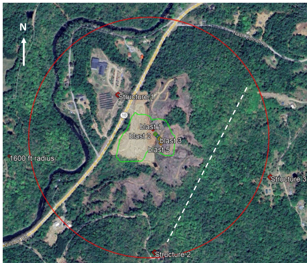
Figure 2. Outline of the Gilsum Quarry permit area (in green) showing the locations of 5 blasts and three structures (Badger Balm, Eaton Hill and Lovell Dr) where seismographs were deployed. The white dashed line indicates an elevated ridgeline 200 ft above the Quarry elevation.
