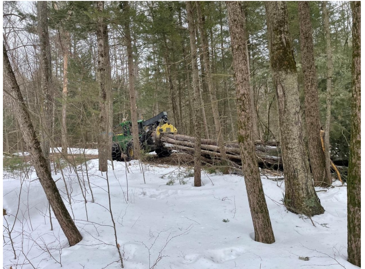
Grapple Skidder pulling a hitch of wood in Walpole, NH this winter
