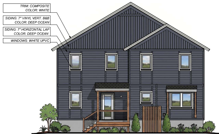
UNIT B UNIT A 1 EXTERIOR ELEVATION STUDY
