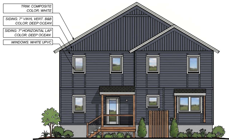
UNIT B UNIT A 1 EXTERIOR ELEVATION STUDY
