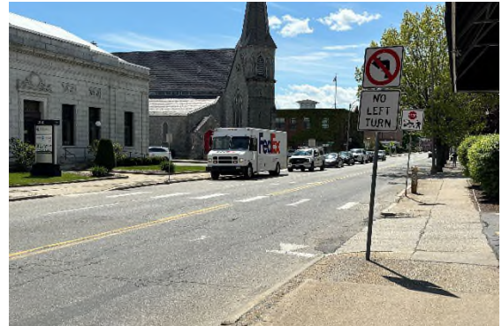
Figure 20. Marked crosswalk on West St., adjacent to the former U.S. Post Office building, crosses three lanes of traffic
